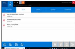
This page instantly displays all the **errors in the vehicle**, with the related codes and descriptions. From this page, the error reading and clearing can be carried out in a single click, as well as a self-diagnosis test on the selected system.
