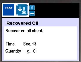
Electronic scales weigh the quantity of oil recovered during services to a high level of accuracy.
