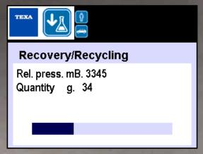
During refrigerant recovery, the display shows the volume of refrigerant recovered and the pressure in the system.
