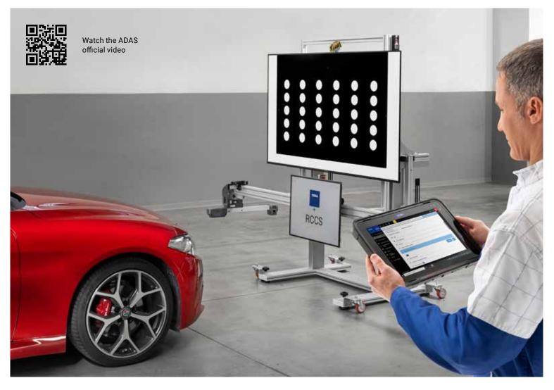
For calibrating sensors, radars, lidars, cameras and sensors TEXA developed and engineered RCCS 3, a top-of-therange solution available in two versions: RCCS 3 with Monitor and RCCS 3 with Panels.
