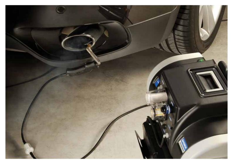
For the checks connected to anti-pollution regulations, TEXA offers tools such as GASBOX Autopower (exhaust gas analyser for petrol and gas vehicles), OPABOX Autopower (opacity meter for diesel engines), MULTI PEGASO 3 (analysis station with a LED monitor), RC2 and RC3 (rev counters for cars and trucks), RCM (rev counter for bikes).
