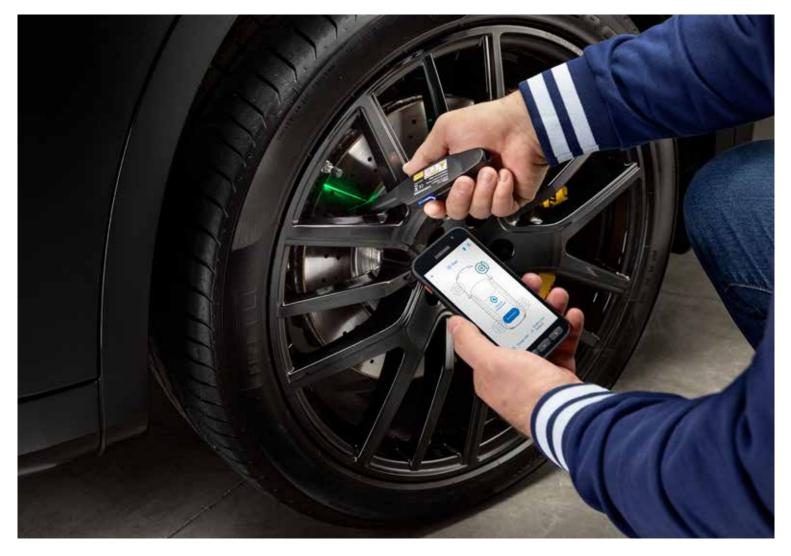
TEXA's new product in the field of measurements is **LASER EXAMINER**, a laser profilometer to check brake disc and tyre tread wear. TEXA's **UNIProbe** and **TwinProbe** interfaces allow taking all the physical measurements required for a conventional diagnosis, identifying potential faults. On the other hand, **TTC** (TEXA TENSION CONTROLLER) is ideal for the correct tensioning and mounting of the timing belt on bikes, ensuring an extremely professional service.
